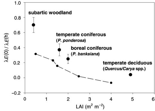
Figure 5. Proportion of total latent heat flux ( $\lambda E(h)$ ) observed at the forest floor ( $\lambda E(0)$ ) increases as leaf area (summer maximum LAI, m<sup>2</sup> half surface area m<sup>-2</sup> ground) becomes more sparse. The dashed line is  $\lambda E(0)/\lambda E(h)$  computed for different LAI values using the CANVEG model (including clumping factors).
