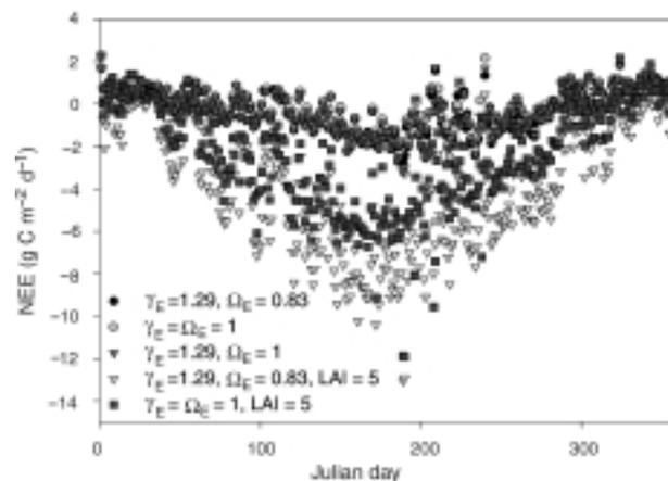
Figure 13. Mean daily net ecosystem exchange (NEE) estimated from CANVEG, based on assuming random distribution of foliage ( $\gamma_E = \Omega_E = 1$ ), clumping at all scales ( $\gamma_E = 1.29$ ,  $\Omega_E = 0.83$ ), and various combinations at measured LAI and at LAI 5. Negative NEE values indicate more net carbon uptake by vegetation. The NEE was affected more than any other variable, and net photosynthesis was affected more at higher leaf areas.
